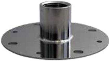
Mounting adaptor (stainless stel) from 140mm flange mount to 1 ¼" -11TPI available
